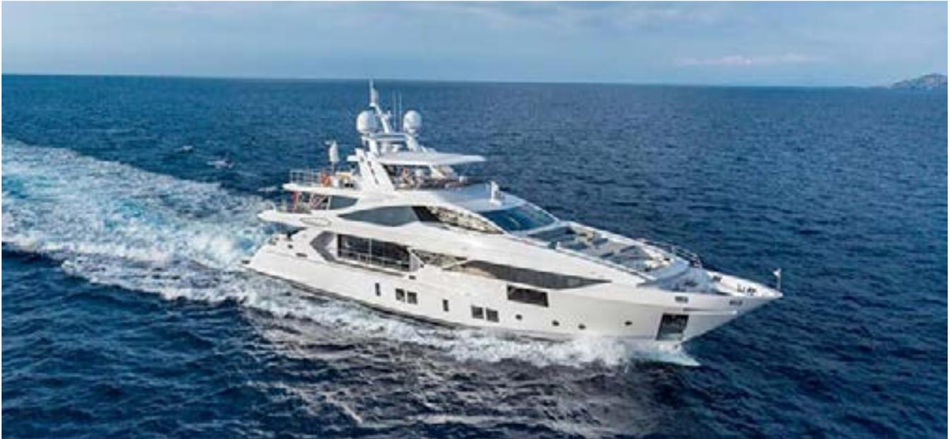
Inspired by the 140' Veloce model, the 125 M/Y Iron Man has a hull measuring 125 feet long and 27.2 feet wide, and a carbon fiber and epoxy superstructure that makes it possible to reduce its weight by 40 percent.
